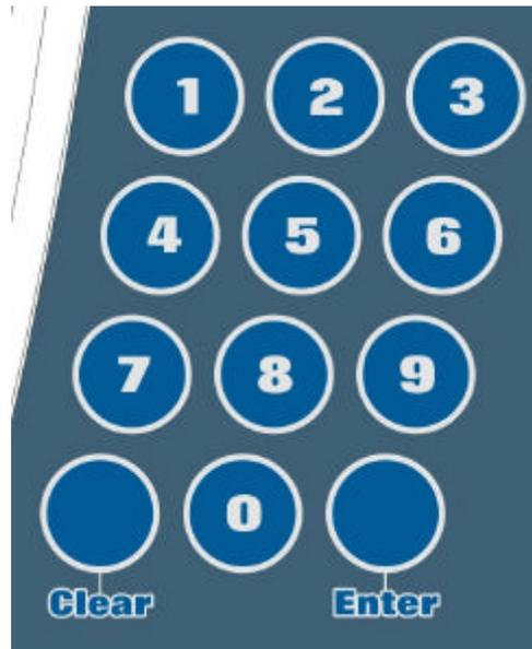
The numeric keypad is located on the right side of the controller. Before the exercise program begins, the numbers are used to enter data in response to the controller prompts. After the workout starts, the numbers are used to enter the desired speed or target heart rate.
