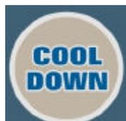
The cool down key will cause the workout program to end. The treadmill incline returns to 0% and the speed decreases to 1.0 MPH if prior speed is less than 2.0 MPH. If the prior speed was greater than 2.0 MPH the speed decreases to 2.0 MPH. You can adjust the incline and speed at any time during the cool down.
