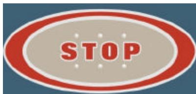
Press the [STOP] key any time you want to pause the workout program for up to one minute. If the [STOP] key is pressed a second time, the workout statistics will be displayed, then the controller will return to the "SELECT WORKOUT" prompt.
