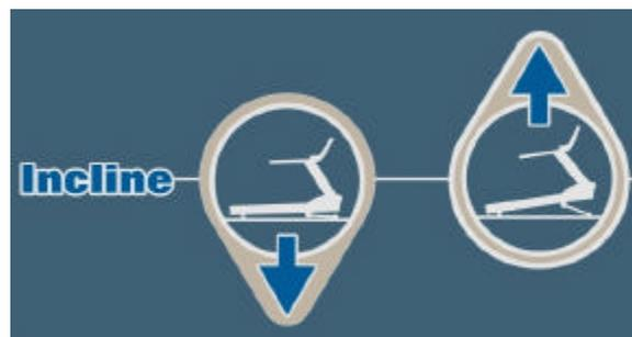
The treadmill incline may be changed at any time during a workout. Pressing the [Incline: ↑] key increases the incline and pressing the [Incline: ↓] key decreases the incline. After the first press of an Incline key, the text line will show the target incline. Further presses will increase or decrease the deck angle by one increment, or 0.5%, depending on the workout option selected.
