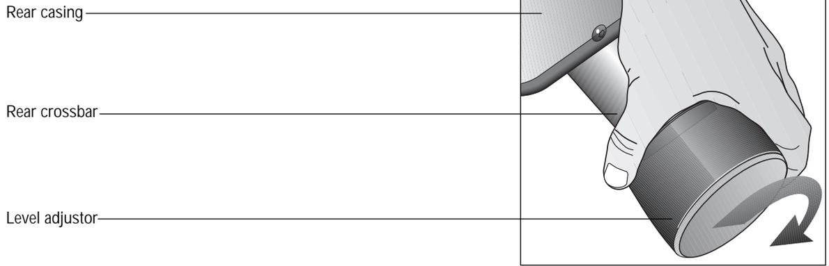
12. If necessary, rotate the level adjustors (on the rear crossbar) so that your unit is level. See Diagram 6.
