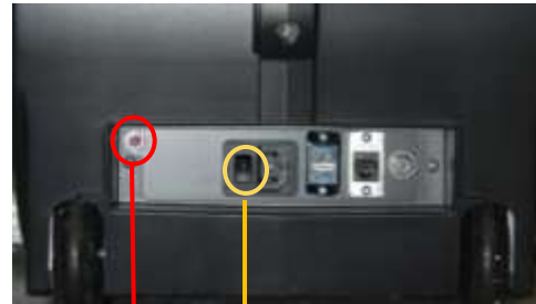
Reset Button Main power switch
