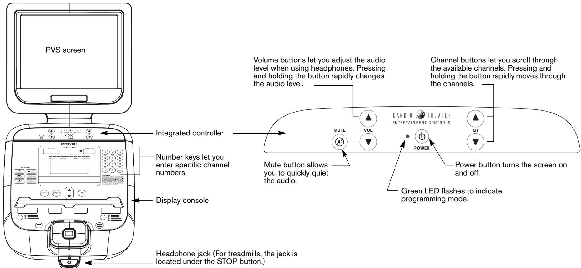
**Figure 1: Overview of PVS screen and integrated controller**
