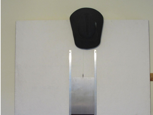
13. Darken Unit with hat or towel (10-60 seconds to initialize motor)
