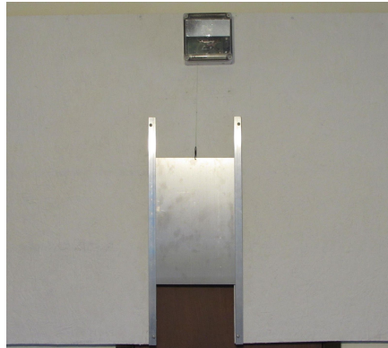
14. Test for smooth opening up after removing darkness.
