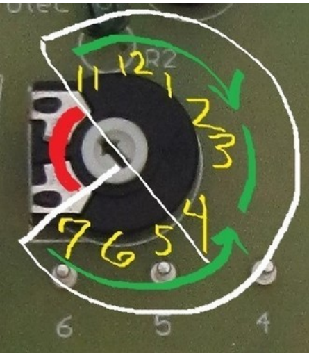
15. Your opener is equipped with a light sensitivity adjustment dial, see the black arrow in the white dial. It is pre-set at the factory for medium sensitivity to daylight. It rotates, from a clock perspective, to the most sensitive to light at 11 o'clock, and the least sensitive to light at 7 o'clock. You can adjust the settings with a small knife tip or a small screw driver, but you must stay within the range of the dial. Never force or crank, it glides smoothly within its range.
