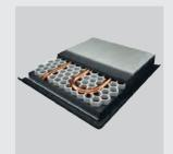
The aluminium honeycomb structure, with its meandering copper pipe, is filled with graphite, enabling heat to be distributed throughout the entire front of the radiator quickly and evenly. Suitable for all low temperature systems, heat pumps, condensing boilers, open or closed heating systems.
