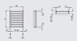
For full **C E** compliant technical specifications, refer to page 140 To make an approximate conversion from T=50K to T=60K multiply outputs by 1.2 \*1/2" air vent Height excludes air vent F = flow
