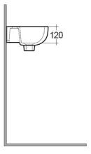
Dimensions: All dimensions in mm tolerance  $\pm 5\%$  for below 200mm and  $\pm 3\%$  for above 200mm. Note: Due to a continuing development programme to improve design and performance, the manufacturer reserves all rights to vary specifications without prior information.
