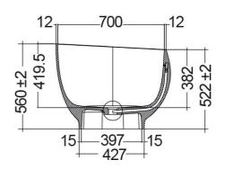
Dimensions: All dimensions in mm tolerance ±5% for below 200mm and ±3% for above 200mm.
