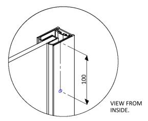
REPOSITION THE INSERT PROFILE AND GLASS ASSEMBLY ONTO THE WALL PROFILE.
