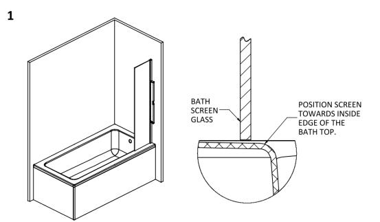
PLACE YOUR BATH SCREEN ONTO YOUR BATH ENSURING THAT THE SCREEN IS TO THE INSIDE OF THE BATH LEDGE AS SHOWN IN THE DETAILED VIEW ABOVE. USE A SPIRIT LEVEL.
