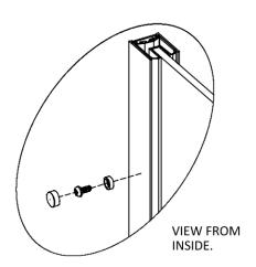
ONCE YOU HAVE MARKED THE POSITION FOR FIXING AND DRILLED THE PROFILE, USE ITEMS 4, 5 & 6 TO FIX THE PROFILE IN PLACE.
