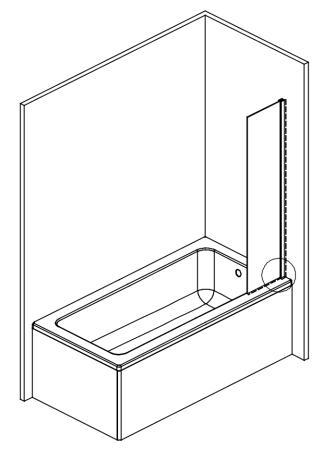
EXTERNALLY SILICONE SEAL THE WALL PROFILE WHERE IT MEETS THE WALL AND ALONG THE BOTTOM WHERE IT MEETS THE BATH. ALL IN A CONTINUOUS BEAD.
