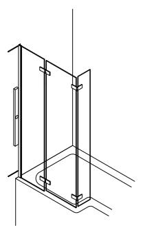
2. PUT THE WALL POST ONTO THE FIXED PANEL, WITH THE HELP OF ANOTHER PERSON PLACE IN POSITION ON THE BATH. USING A SPIRIT LEVEL MARK THE POSITION OF THE WALL POST ON THE WALL WHERE IT WILL BE FIXED.
