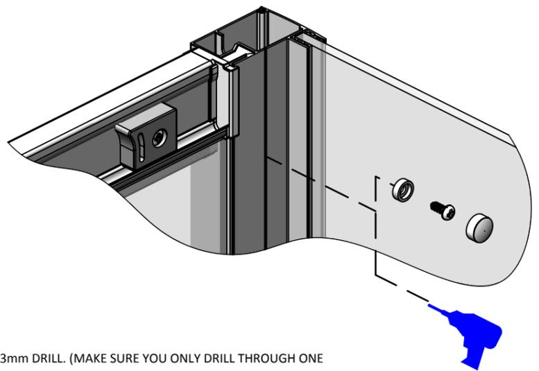
WHEN THE ENCLOSURE IS READY TO BE FIXED, DRILL THROUGH THE HOLES IN THE WALL PROFILE AND CORNER POST WITH A 3mm DRILL. (MAKE SURE YOU ONLY DRILL THROUGH ONE WALL THICKNESS) THEN FIX THE FRAME WITH ITEMS 4, 5 & 6.
