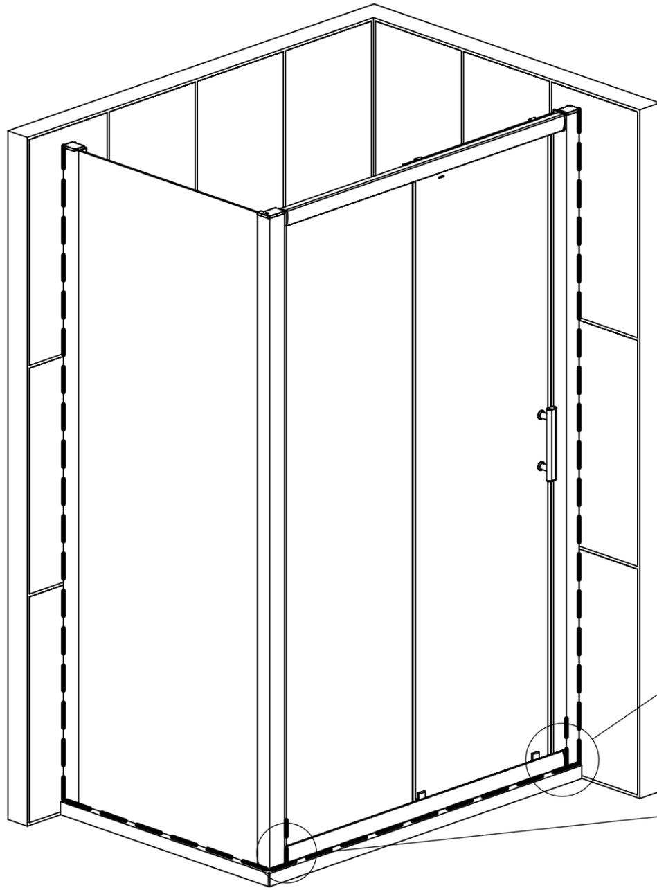
EXTERNALLY SILICONE SEAL THE WALL PROFILES WHERE THEY MEET THE WALL AND THE BOTTOM PROFILE AND GLASS SIDE PANEL WHERE IT MEETS THE TRAY. ALL IN A CONTINUOUS BEAD.
