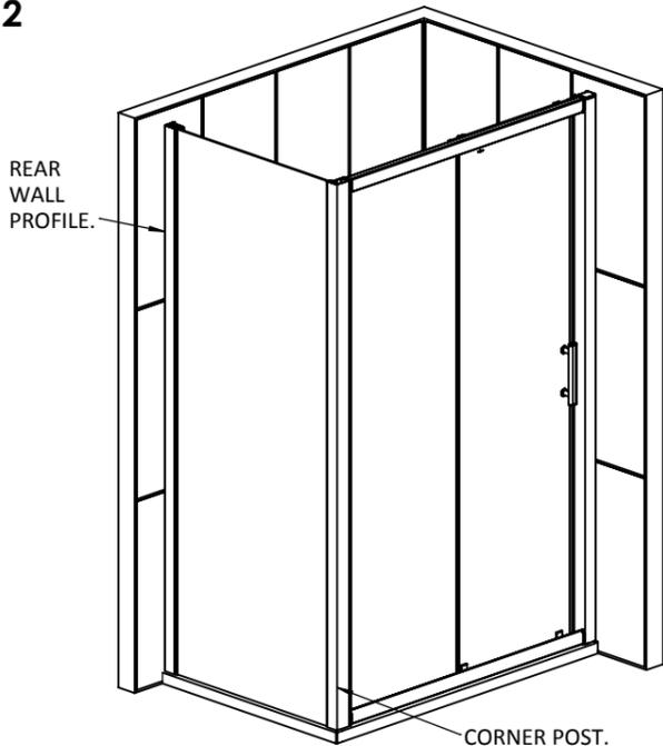
HOOK THE SIDE PANEL CORNER POST ONTO ENCLOSURE THEN SLIDE THE SIDE PANEL INTO REAR WALL PROFILE.
