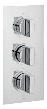
**DESCRIPTION:** DX Notion concealed 2 outlet, 3 handle thermostatic shower valve wall mounted with rectangular backplate thermostatic cartridge V-001C-PLA flow cartridge C-301-RTC 2 x 3/4" female inlets 2 x 3/4" female outlets includes 3/4" - 1/2" adaptors inc. bleed valve for system flush on installation min-max wall mount 70-95mm optimum installation depth 82mm minimum operating pressure 0.2 bar LP (shower) minimum operating pressure 1.0 bar MP (bath)
