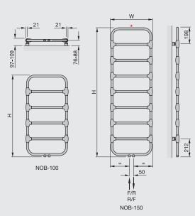
\*1/2" air vent (rear) F = flow R = return H = height W = widthTube: O 25mmAll dimensions in mm
