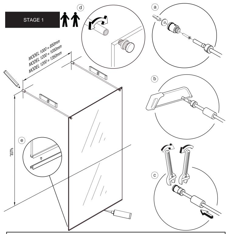
We recommend two people are available. Using a level, plumb and mark the centre of the Wall plate on the wall. As a guide measure 2079mm up from the finished floor surface and see dimension above for the dimension between centres relative to Model.
