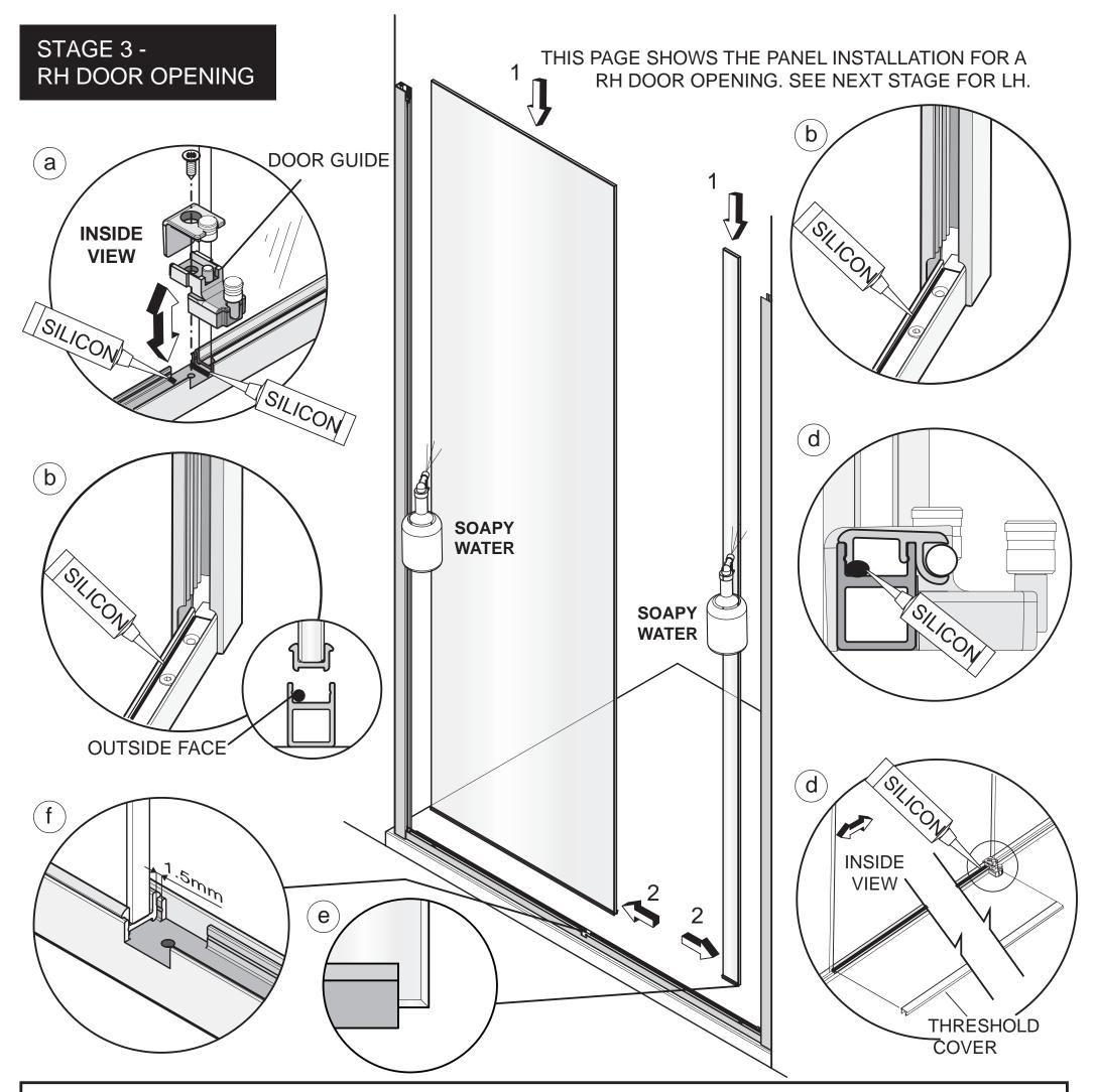
This stage is describing the fitting of the Fixed panel and Closure panel, for a RH Door opening, see next page for LH Door opening. Before fitting the fixed glass panel adjust the threshold extrusion so that it is equally positioned between the two wall mounts. Loosen the threshold adjusters at each end and lightly tighten in position as required.
