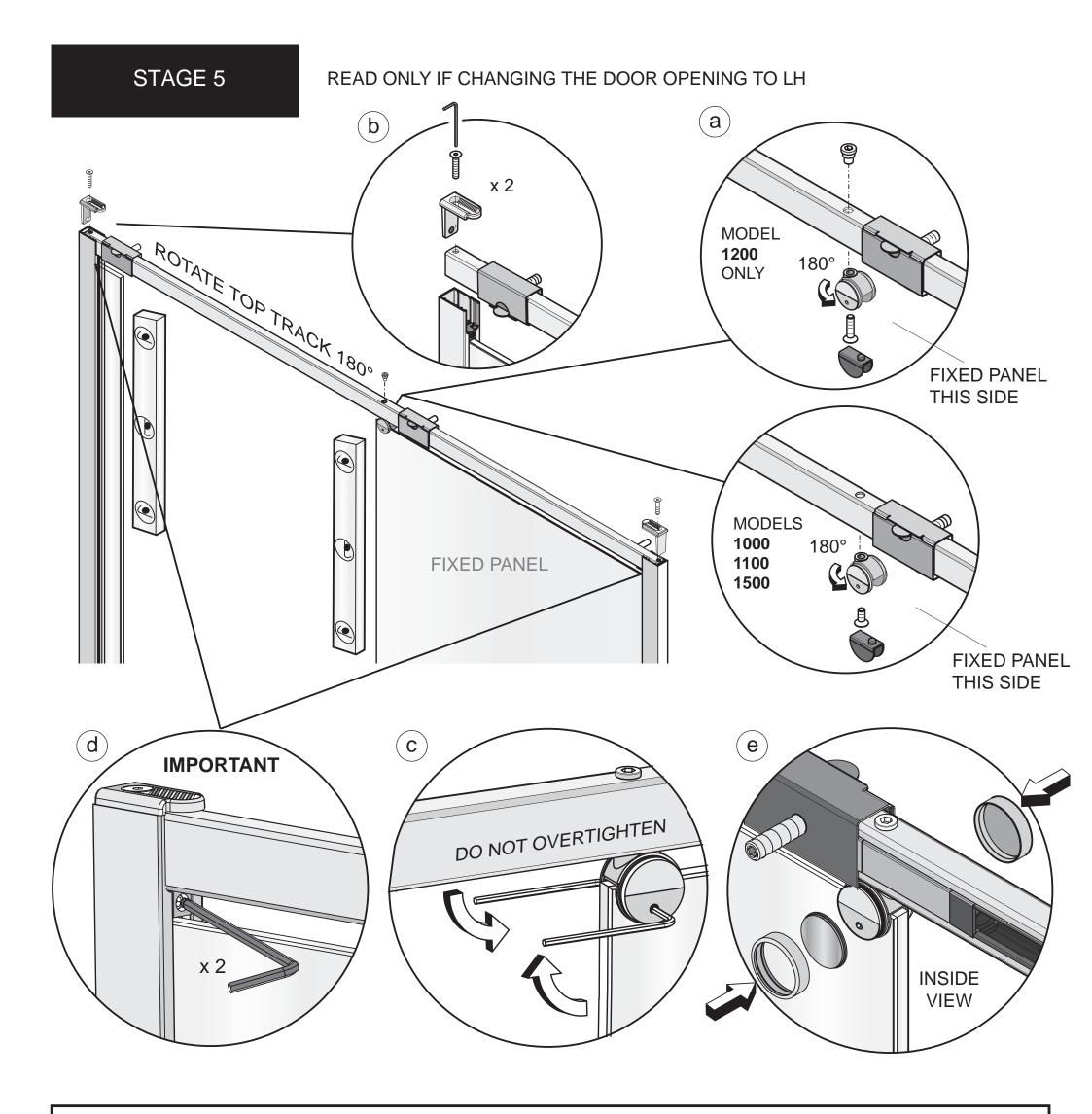
This stage is describing how to reverse the top track to a LH door opening and the fitting of the Top Track.
