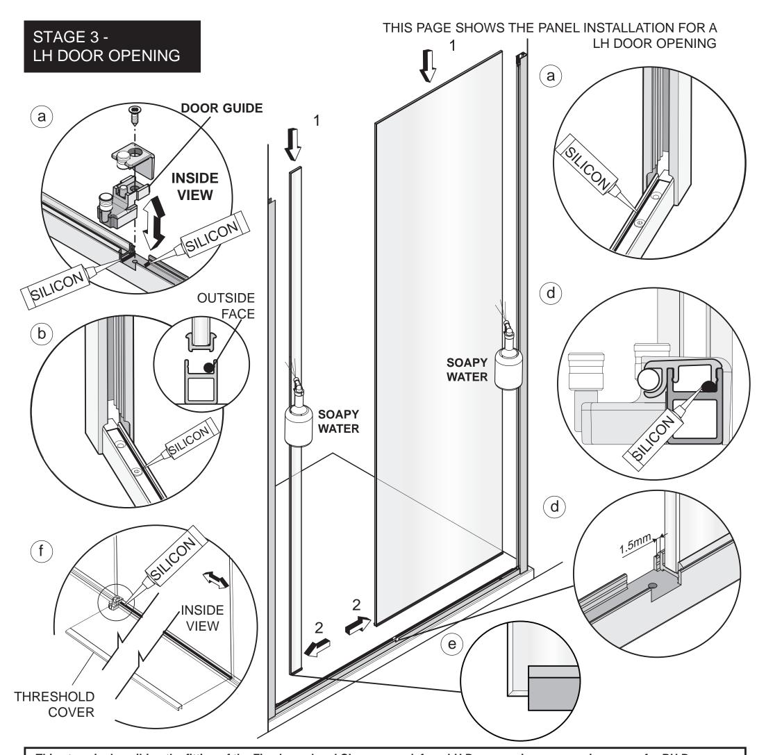
This stage is describing the fitting of the Fixed panel and Closure panel, for a LH Door opening, see previous page for RH Door opening. Before fitting the fixed glass panel adjust the threshold extrusion so that it is equally positioned between the two wall mounts. Loosen the threshold adjusters at each end and lightly tighten in position as required.
