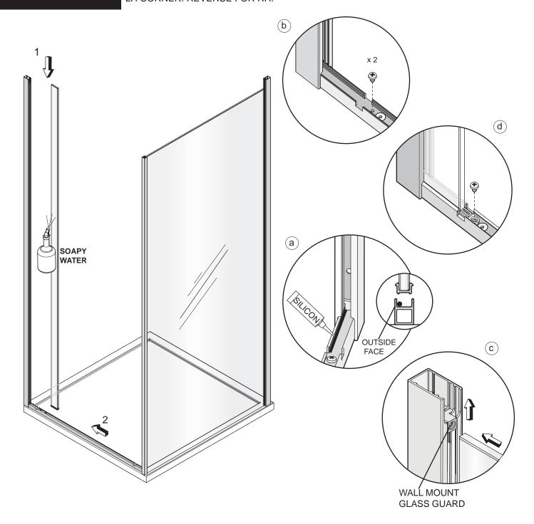
This stage is describing the fitting of the fixed panel for a LH Corner, reverse for RH Corner. Before fitting the fixed glass panel adjust the threshold extrusion so that the side panel is at right angles to the threshold extrusion. Loosen the threshold adjuster and lightly tighten in position as required.
