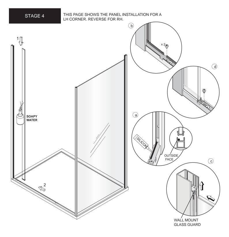
This stage is describing the fitting of the fixed panel for a LH Corner, reverse for RH Corner. Before fitting the fixed glass panel adjust the threshold extrusion so that the side panel is at right angles to the threshold extrusion. Loosen the threshold adjuster and lightly tighten in position as required.
