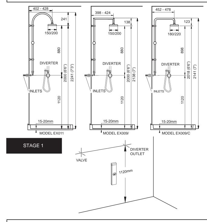
This stage is describing the positioning of the Diverter for models EX009, EX009/C and EX011.
