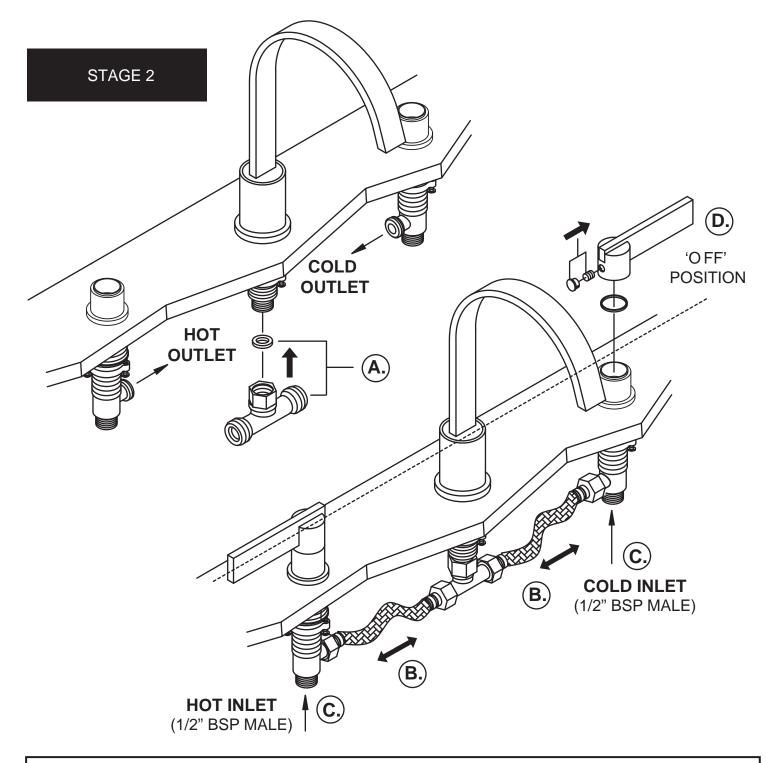
This stage describes connecting the Taps and Spout with the hot and cold water supplies.
