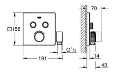
Product Description: GROHTHERM SMARTCONTROL Thermostat for concealed installation with 2 valves and integrated shower holder
