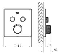
Product Description: GROHTHERM SMARTCONTROL Thermostat for concealed installation with 2 valves
