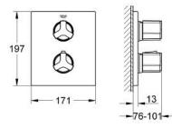
Product Description: ALLURE Thermostat with integrated 2-way diverter for bath or shower with more than one outlet
