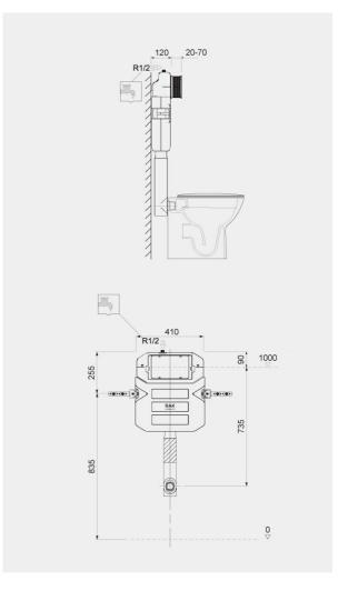
Dimensions: All measurements are in millimeters and are subject to normal manufacturing variations.
