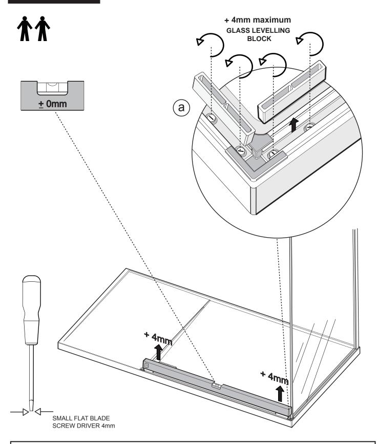
This stage is describing the fitting of the Corner Front panel.
