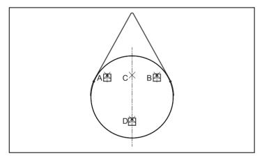
2.Measure the distance between centre of hanging holes in bracket A and B. Find the mid-point C of line segment AB. Measure the distance between C and the centre of bracket D.
