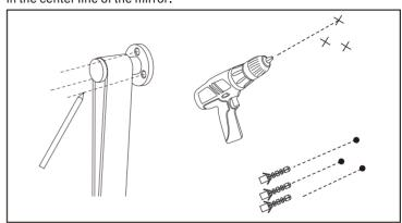
6.Use a pencil to mark the positions through the holes in the hook bracket, use a power drill and 6mm drill bit to drill holes. Use hammer to insert the wall plugs.
