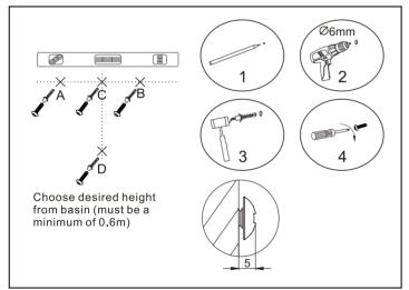
3.Choose desired height from basin (must be a minimum of 0.6m). Use a pencil to mark the positions of A, B, C, D according to the measured sizes. A, B, D are the positions for the 3 screws. Use a power drill and 6mm drill bit to drill holes. Use hammer to insert the wall plugs. Use screwdriver to tighten the screws. Note: The distance between wall and the top of screw head should be 5mm.
