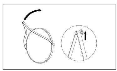
5.Place the hook bracket behind the loop of the strap, lift the strap up against the wall and ensure the hook bracket is at the highest position in the center line of the mirror.
