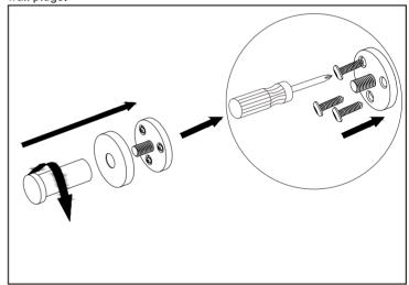
7.Insert screws through the hook bracket and fasten in place. Once secure, place the cover over the bracket and screw on the hook.
