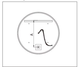
2. Measure distance A between center of hanging hole and hanging bar.
