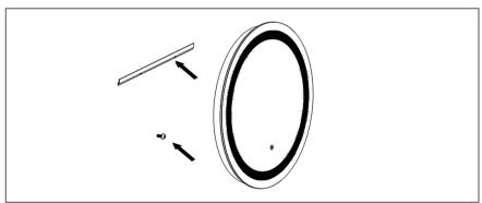
5. Hang the mirror onto the wall. Shake left and right to see if it is stable.
