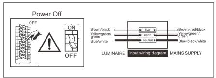
4.Make the electrical connections ensuring first that the electrical supply has been turned off. This mirror is a class 1 product and requires an earth connection. It should be installed in accordance with the latest IEE regulations.
