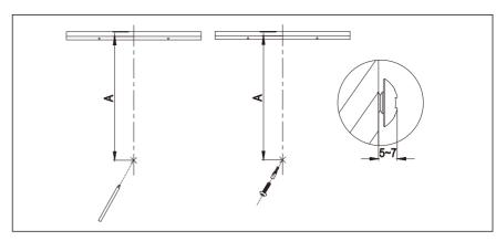
3.On the centre line of the hanging bar, measure distance A from the centre of the hanging bar as above. Use a pencil to mark the position. Use hammer to insert the wall plug. Use screwdriver to tighten the screw.
