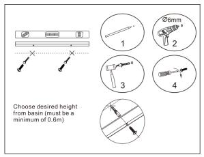
1.Choose desired height from basin (must be a minimum of 0.6m). Use a pencil to mark the positions through the hanging bar hole. Use a power drill and 6mm drill bit to drill holes. Use hammer to insert the wall plugs. Use screwdriver to tighten the screws.
