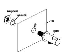
Step 1: Select a proper position on the tile and drill a hole of Ø25mm with depth of 110mm. Fix the valve into the wall. Mount the body with washer and backnut. Connect inlet with valve body and check for leakage.
