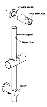
Step3: Place the sliding rail into the valve body. Keep the rail side with bigger hole at the front, and place wall bracket and cover plate against the wall. Finally place sliding rail.
