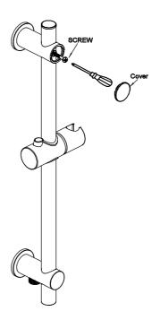
Step4: Fix the sliding rail and wall bracket together against the wall with screw, tighten with a screw driver through the bigger hole in the sliding rail and place cover.
