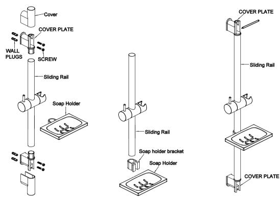
Step 1: Disassemble all the parts according to the figure above.
