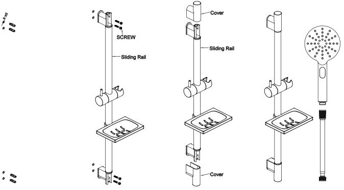
Step4: Drill two holes of Ø6mm with depth of 40mm.Tap in wall plugs.
