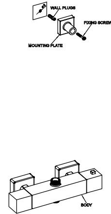
Step 5: Place mounting plate against wall and make markings for a hole. Drill a hole of 26mm with depth of 45mm. Tap in wall plugs, then fix the mounting plate against wall with screws.
