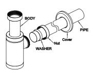
Step2: Put washer, nut and cover on the pipe, then connect pipe to the body.
