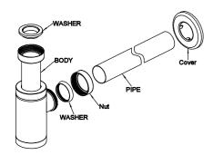
Step 1: Disassemble all the parts according to the figure above.
