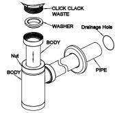
Step3: Loosen the nut, and then pull the body to adjust up and down, so that the outlet of the body is in line with the drainage hole. Insert the pipe into the drainage hole, put the washer into the body, install it on the click clack basin waste, and then tighten the seal.
