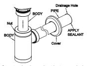
Step4: Apply sealant between drainage hole and pipe, tighten the nut. After the sealant solidifies, pour the water into the basin for drainage, test for water leakage, and finally install the decorative cover on the wall.
