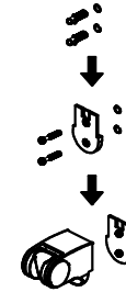
Step 5: Drill a hole of 6mm with depth of 40mm, tap in wall plugs. Fit the mounting plate on the wall with screws. Finally fit handset holder against wall.
