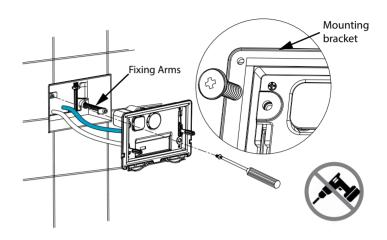
Re-connect the clip links and cable ribbon to the glass fascia and insert the battery holder. Place the front glass plate and remove the protective film prior to testing its functioning. Once correctly attached the flush plate will illuminate for a couple of seconds.
