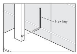
Secure riser in position using the grub screw on the underside of the bracket.
