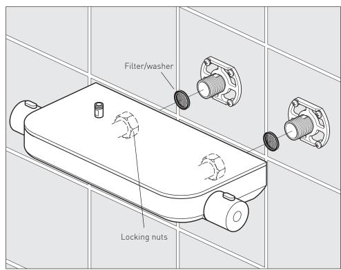
Place a rubber filter/washer in each of the locking nuts on the valve and screw onto the connectors.
