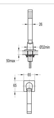
Dimensions are in millimetres except thread sizes which are BSP imperial.
