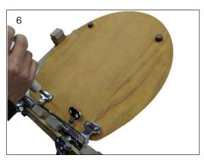
Place the soft hinges as shown in below image, and fit them onto the lid by screws provided. Fix the screws into the plastic inserts.
