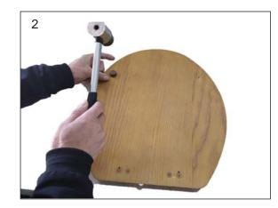
Assemble two small round buffers onto the lid. Use plastic hammer to fit the small round buffers into pre-drilled holes if needed.
