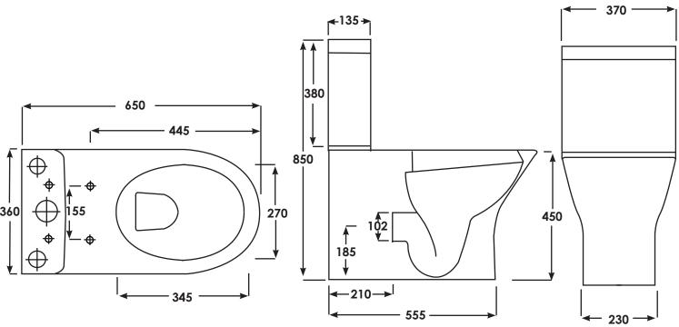
Dimensions: All measurements are in millimeters and are subject to normal manufacturing variations.
