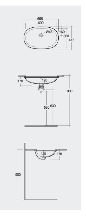
Dimensions: All dimensions in mm tolerance  $\pm 5\%$  for below 200mm and  $\pm 3\%$  for above 200mm. Note: Due to a continuing development programme to improve design and performance, the manufacturer reserves all rights to vary specifications without prior information.
