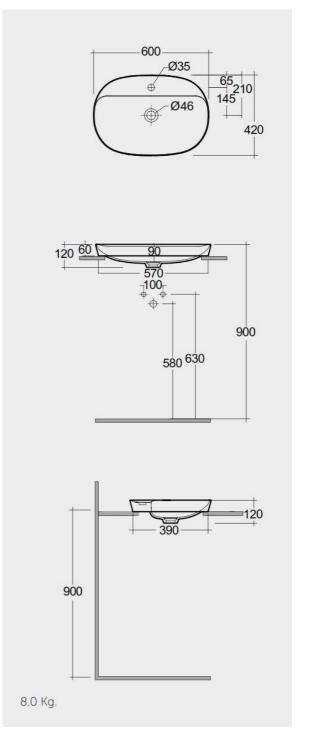
Dimensions: All dimensions in mm tolerance  $\pm 5\%$  for below 200mm and  $\pm 3\%$  for above 200mm. Note: Due to a continuing development programme to improve design and performance, the manufacturer reserves all rights to vary specifications without prior information.
