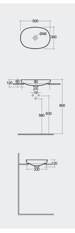
Dimensions: All dimensions in mm tolerance ±5% for below 200mm and ±3% for above 200mm. Note: Due to a continuing development programme to improve design and performance, the manufacturer reserves all rights to vary specifications without prior information. Please note accessories are for photographic use only.
