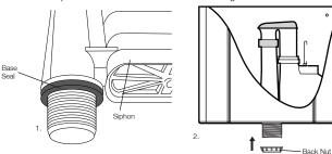
Once the outlet valve is assembled in the cistern, keeping hold of the piston, remove the tie wrap. Once this has been removed, install the C-link to the piston. To make the installation easier, the piston may need to be pushed upwards from the underside.
