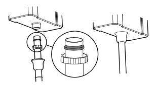
3. Insert the flush pipe into the bottom of the cistern and tighten the compression fitting. To ensure a good seal use PTFE tape, around the thread.
