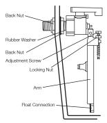
Screw the float into the swivel arm screw and assemble inside the cistern tank as shown. Check for free movement of the float (ensure the float does not get caught on the side/back wall of the cistern). To adjust the water level rotate the water level adjustment screw. Turn clockwise to reduce shut-off level, turn anti-clockwise to raise shut-off level, secure by hand tightening the locking nut.
