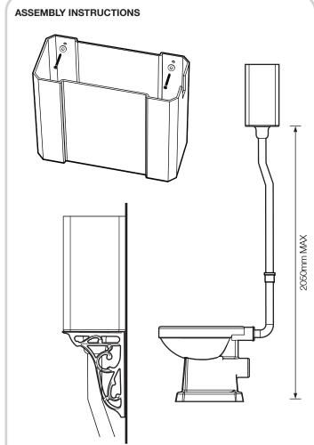
1. The underside of the cistern can be a maximum of 2080mm off the floor.
