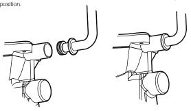
4. Insert the flush pipe and flush cone into the inlet hole on the pan. Ensure the pipe is fitted securely into the pan.
