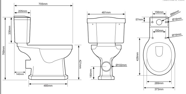
What side is the inlet located? Right hand side of cistern.
