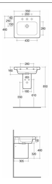
Dimensions: All dimensions in mm tolerance ±5% for below 200mm and ±3% for above 200mm.
