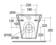
Dimensions: All dimensions in mm tolerance  $\pm 5\%$  for below 200mm and  $\pm 3\%$  for above 200mm. Note: Due to a continuing development programme to improve design and performance, the manufacturer reserves all rights to vary specifications without prior information.
