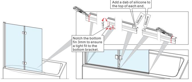
11. Fix the luna rail on top of bath. Put a dab of silicone to bottom of each luna rail end cap (note left & right) and a thin bead of silicone to the bottom of the luna rail. Fit cap to end of fixed panel and carefully place luna rail into end cap. Ensure the luna rail is parallel to the bath edge. **Fig 11.**
