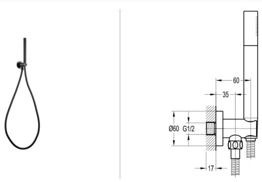
Dimensions are in millimetres except thread sizes which are BSP imperial.
