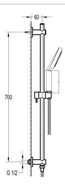
Dimensions are in millimetres except thread sizes which are BSP imperial.
