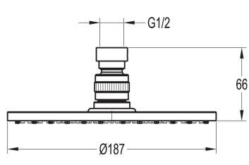
Dimensions are in millimetres except thread sizes which are BSP imperial.
