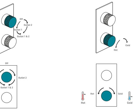
Turning the flow control handle in the direction of the arrow increases the flow of water to the outlet.
