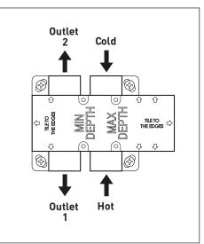
Finish the wall by tiling up to the mortar guard, keep the final finished wall surface between the min and max marks.
