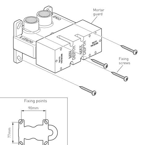
Select the position for the shower valve and offer the shower valve to the wall, make sure the valve is horizontal with a level and mark the 4 fixing points with a suitable pencil, see above left for dimensions. Remove the shower valve from the wall, drill the holes to a suitable depth for the wall plugs and secure with suitable screws. Installation
